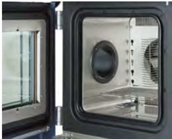
Left side \phi 100 Cable port (option)
