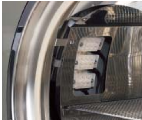
Signal terminals inside chamber
